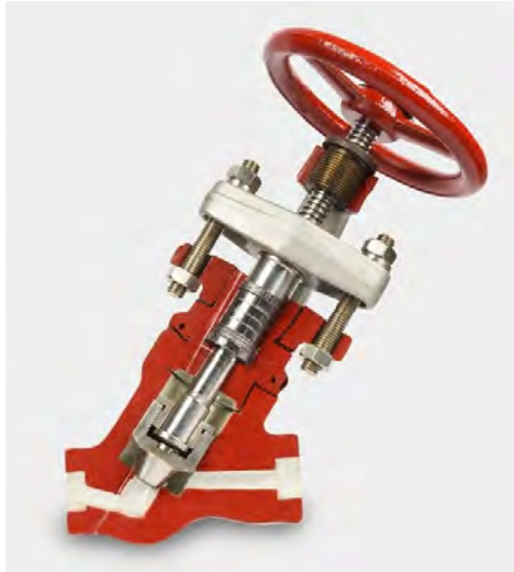
รูปที่ 3-18 Y-Body Design Socketweld End, Bolted-Bonnet, Outside-Screw-and-Yoke, Spherical Disc, Globe Valve
