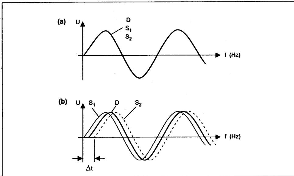
**Sine Waves, (a) No Flow, (b) Mass Flow**
