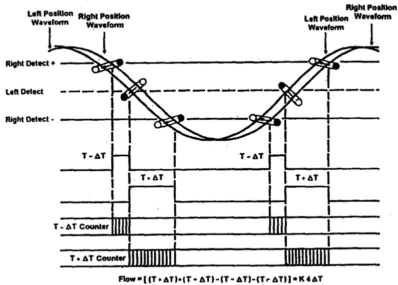
RFT9739 Detection of Flow Tube Phase Shift ( $\Delta T$ )
