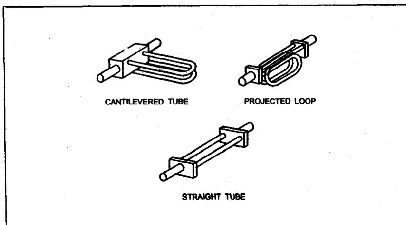
**Coriolis Flowmeter Flow Tube Configurations**
