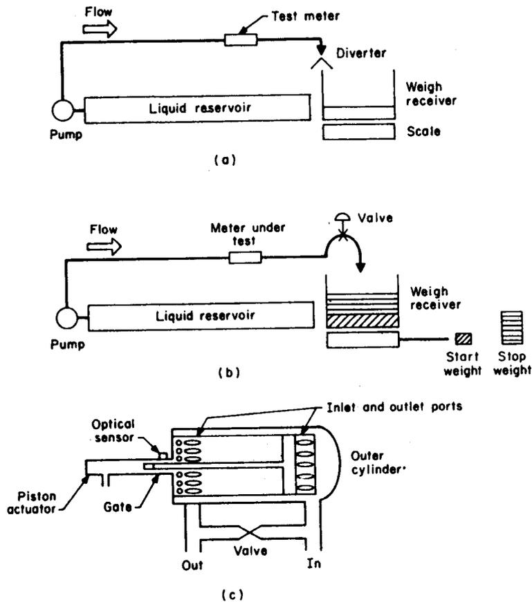
Liquid calibration standards. (a) Static weighing. (b) Dynamic weighing. (c) Ballistic prover.
