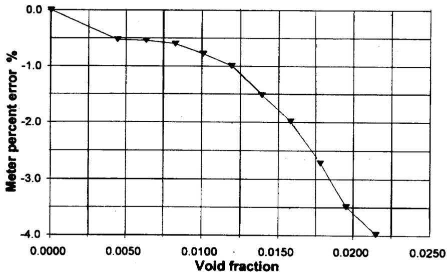
Figure Effect of bubbly flow on a Coriolis mass flowmeter.
