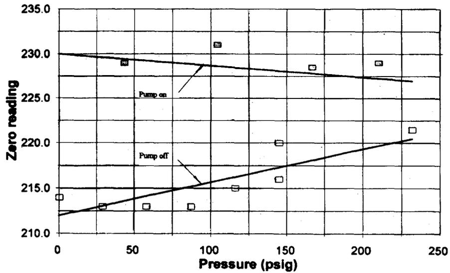
Figure Effect of pressure of the zero of a Coriolis mass flowmeter.
