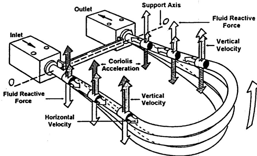
**Flow Tube Response to Coriolis Acceleration**
