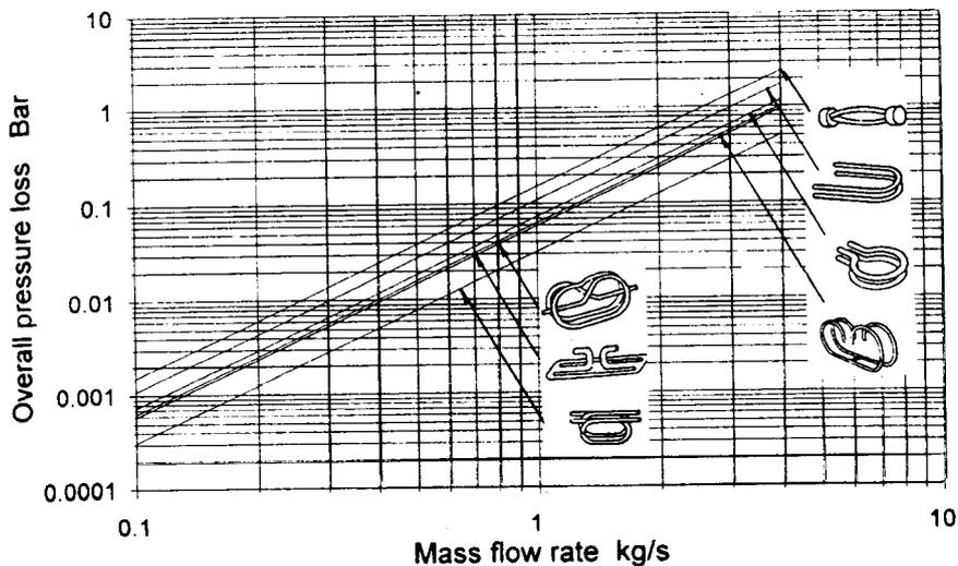
Figure Overall pressure loss for a 1 in (25 mm) Coriolis mass flowmeter.
