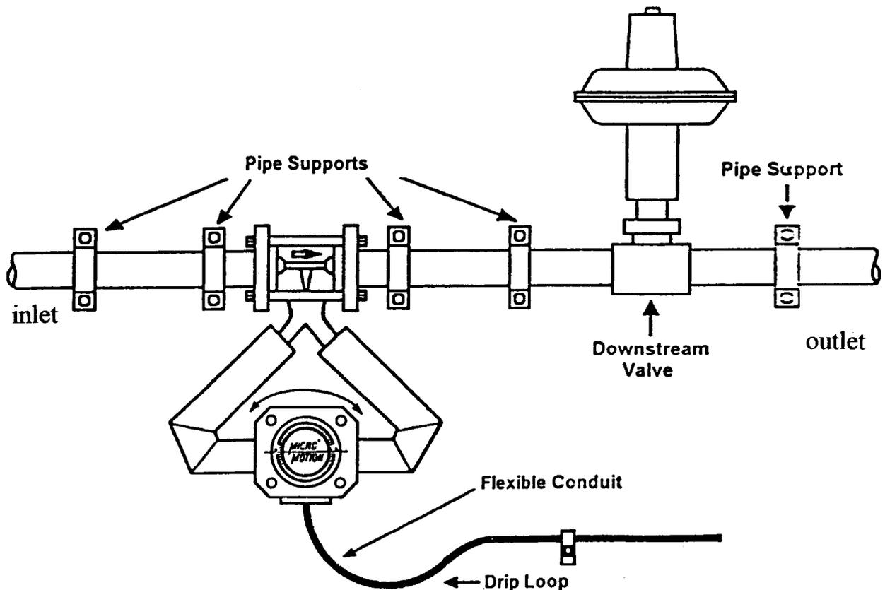
Recommended Sensor Installation in Process Piping
