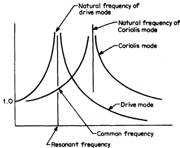
Figure Coriolis and drive mode frequency relationships.
