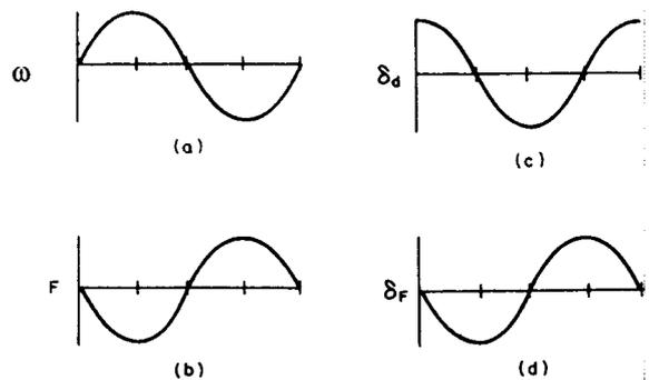
Coriolis frequency and displacement relationships. (a) Angular frequency. (b) Force. (c) Drive displacement mode (d) Force displacement mode.
