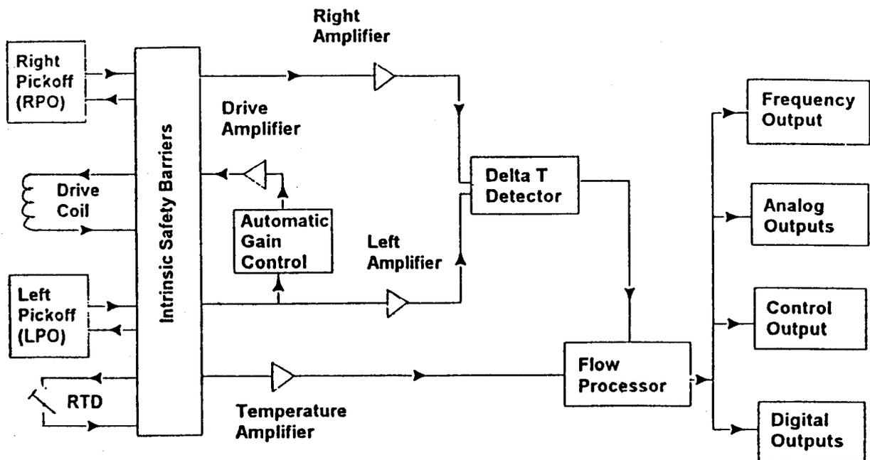
**Remote Flow Transmitter Signal Processing Diagram**
