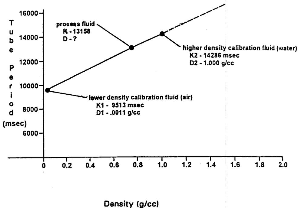
Determining Process Density on the Basis of Reference Densities
