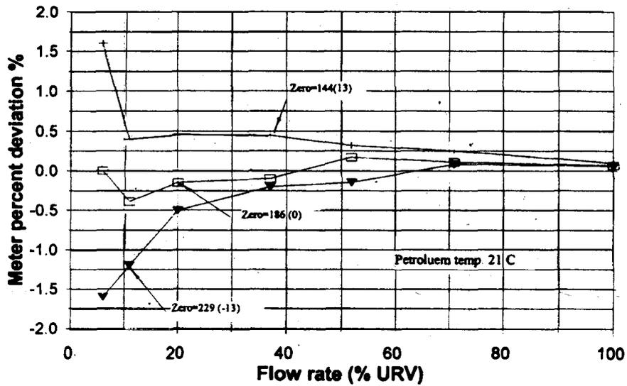
Figure Effect of zero on the calibration curve for a Coriolis mass flowmeter.
