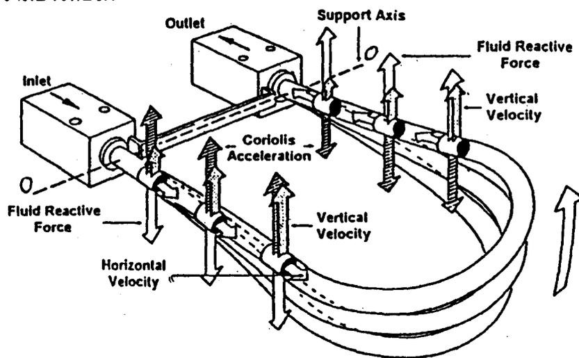
Flow Tube Response to Coriolis Acceleration
