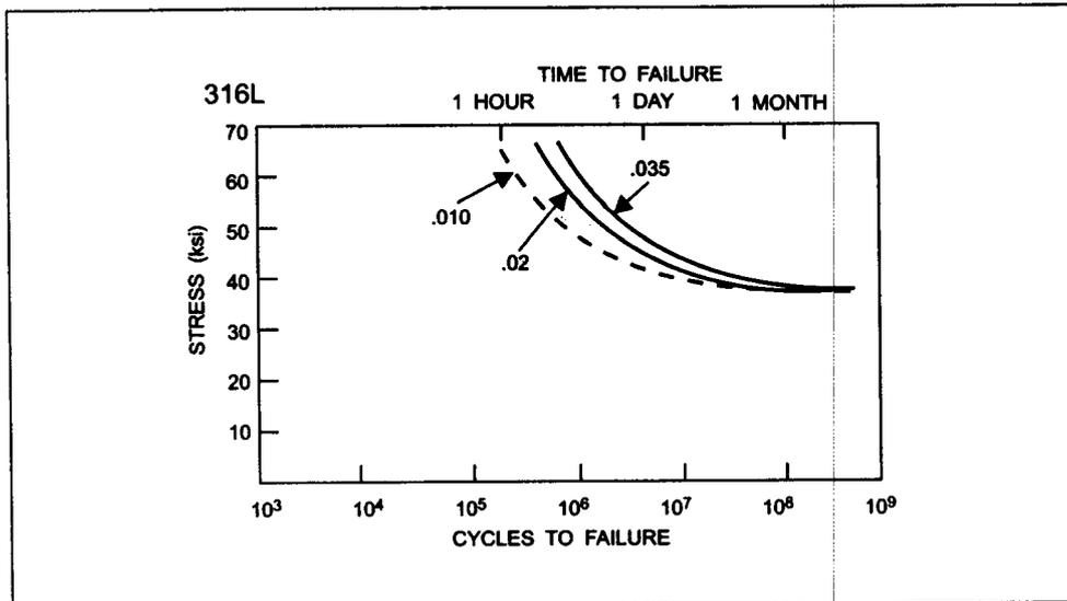
Endurance Characteristic Curves for Various Wall Thicknesses of Tubing
