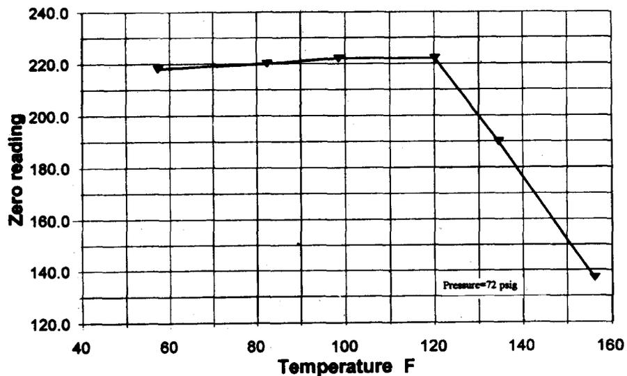
Figure Effect of temperature on the zero of a Coriolis mass flowmeter.
