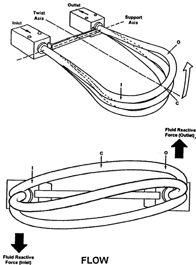
**Oscillating Flow Tube, Response to Flow**
