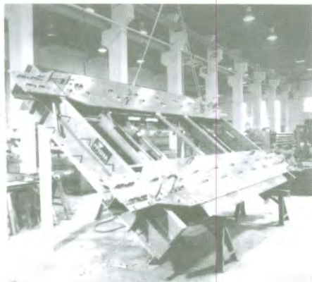
Low-profile rail wa- gon weighbridge in the factory
