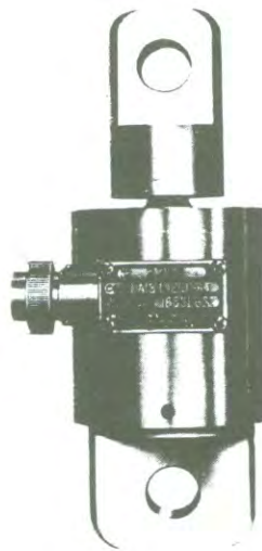
Figure Induction load cells range in size from 1½ inch diameter by 2½ inches long for 600-pound capacity to 6¾ inch diameter by 10¾ inches long for 300,000-pound capacity. Cell shown is for tension measurement. (Courtesy of W.C. Dillon and Company, Inc.)
