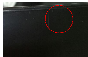
After improvement (weld line length is 7.23 mm)
